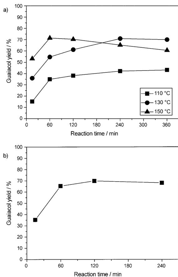
**Figure 2.** a) The effect of reaction temperature on cleavage of the  $\beta$ -O-4 bond of GG; b) cleavage of the  $\beta$ -O-4 bond of VG at 150 °C.
