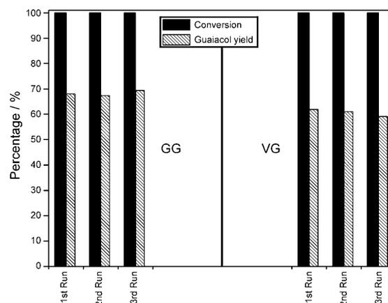
**Figure 6.** Recycling tests on cleavage of the  $\beta$ -O-4 bonds of GG and VG in [HMIM]Cl.
