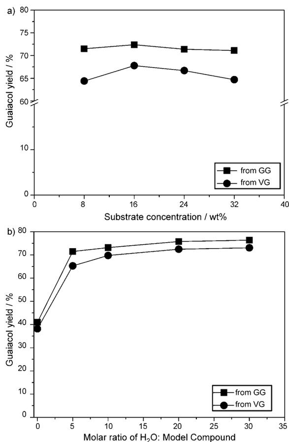
**Figure 5.** a) The effect of substrate concentration on cleavage of the  $\beta$ -O-4 bonds of GG and VG; b) the effect of water concentration on cleavage of the  $\beta$ -O-4 bonds of GG and VG.
